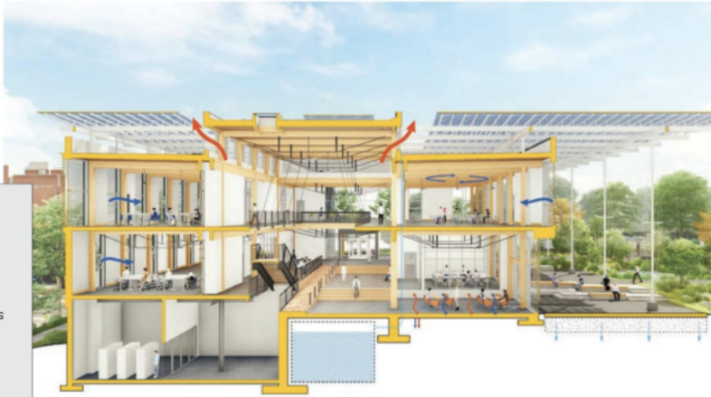
Operable windows and 60+ ceiling fans maintain comfortable airflow throughout this Atlanta-based building.
